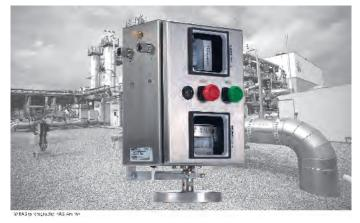
Safety Equipment for Natural Gas Extraction (ATEX, SIL) | To replace an expensive setup with several instruments and components PINTER was asked to developed a unique system to control gas extraction with regard to MAX and MIN pressure monitoring, supply air control, batterypowered GSM-alarm and many other functional and safety-related features.
