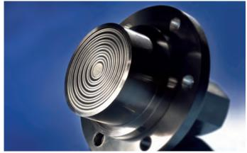
**Diaphragm Seals** | Mechanical process separating elements which are mounted on measuring instruments directly or via capillary; with diaphragm seals the measuring instrument is separated from the actual process to protect the instrument from hot, polluted, aggressive or chrystalizing media.
