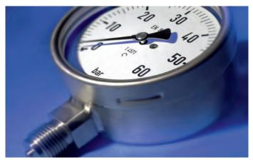
**Pressure Gauges** | Mechanical pressure indicators. The actual process pressure acts on a measuring element and deforms it. The deformation is converted into a 270° rotating motion by the attached movement. Due to the electricity-free function, pressure gauges even remain fully functional in most total damage occurance.
