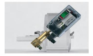
**Special Design Pressure Switch (TÜV)** | This specially designed unit used on MRTs is able to switch 13 mbar on failing helium supply plus it withstands overpressure shocks up to 4 bar without any malfunctions. The integr. pressure transdcuer is used for signalling to a PLC and the integr. pressure gauge tells the service personell if the system is pressurized even when there is no power supply.
