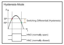
In Hysteresis-Mode both switching point SP and reset point RP can be adjusted freely. The switch switches back when the RP is reached. This allows, for example, a simple 2-point control.
